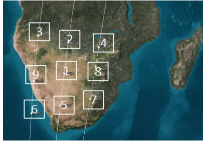
Figure 65: Eight available differential RAAN-TA slots (exact values in Table 10) arranged around the reference satellite (+1), as enumerated in an AGI-STK simulation.
