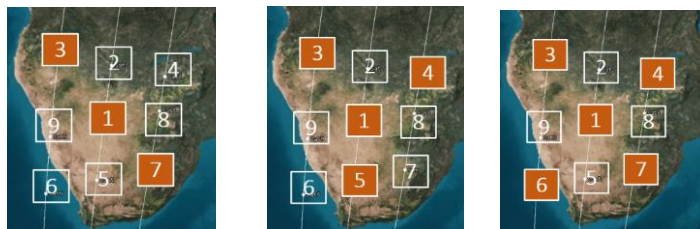
Figure 132: [Left] Arrangement of the 3-sat formation (orange) in the 9 given slots (white) corresponding to maximum BRDF and albedo errors in Table 21 (also highlighted in orange) when sorted by BRDF in either chief orbit. [Center] 4-sat formation arrangement (orange) for minimum errors, when sorted by albedo, in either orbit. [Right] 5-sat formation arrangement (orange) for minimum errors when sorted by BRDF. The orbit of Sat#1 is the chief orbit, flanked by two others with \Delta\Omega = 5\text{deg} on its sides.
