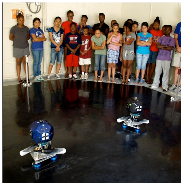
Figure 27: A 3 Degree of Freedom (DOF) test using two SPHERES satellites on the MIT Flat Floor Facility. The onlookers are middle school students participating in the Zero Robotics Summer of Innovation Program 2010 for middle school students in the greater Boston area
