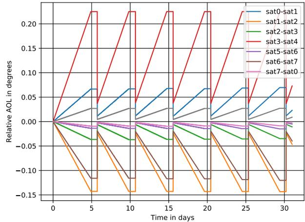
**Figure 6:** GMAT simulation results: The relative AOL drift between eight consecutive satellites of the CYGNSS constellation, and phasing maneuvers that correct for the drift when a 0.5% threshold is breached.
