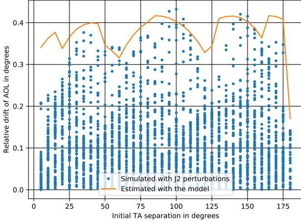
(a) Inclination of  $36^\circ$  and altitude of 378 km. Twelve orbital planes with six satellites per plane.
