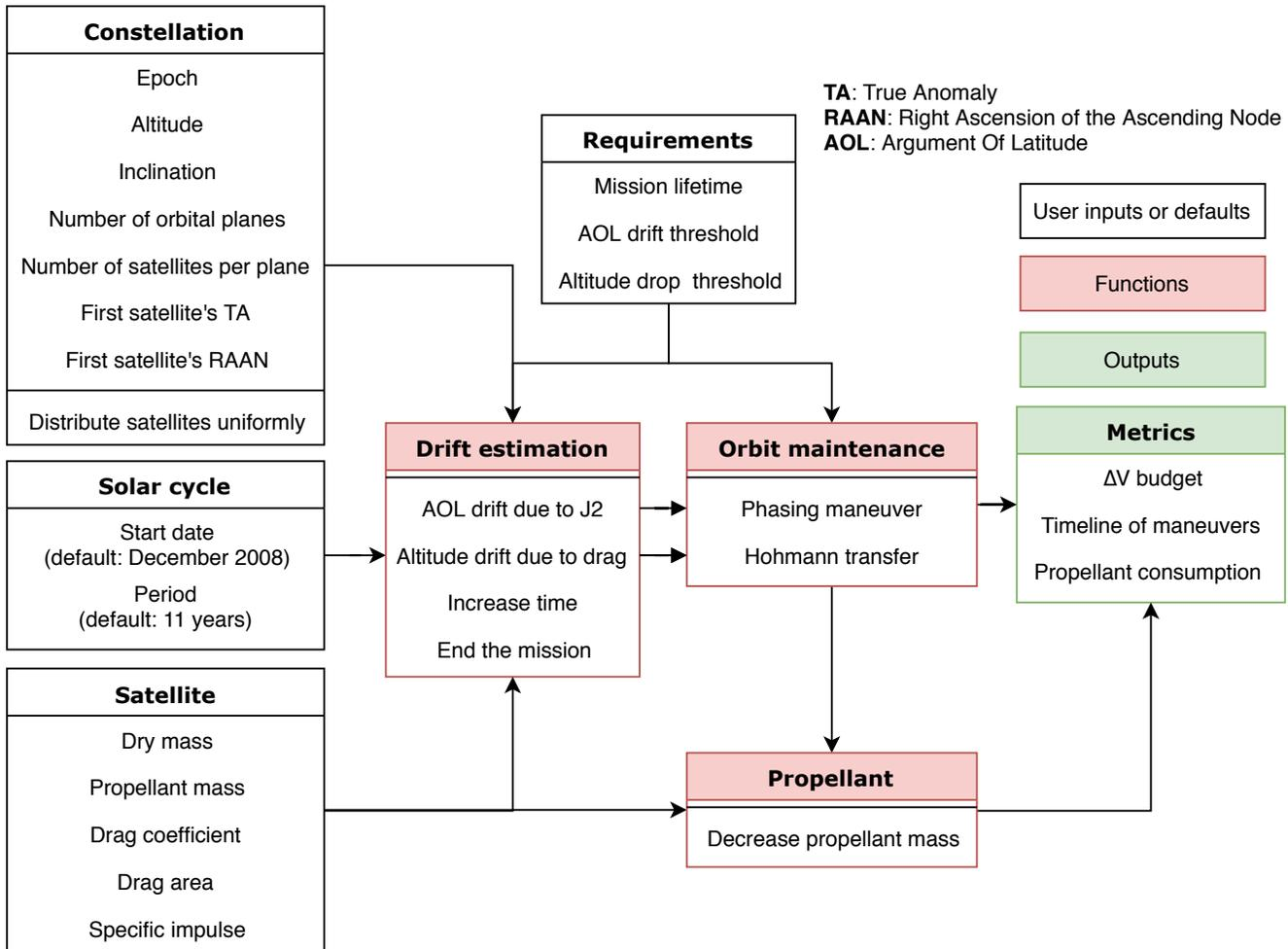
Figure 5: Information flowchart for the Orbit Maintenance Module.
