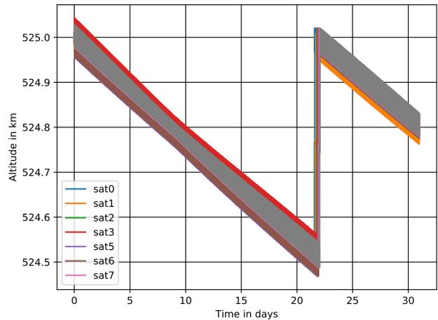
**Figure 7:** GMAT simulation results: The altitude drift of eight satellites of the CYGNSS constellation, and Hohmann transfers that raise orbits when a 0.1% threshold is breached.
