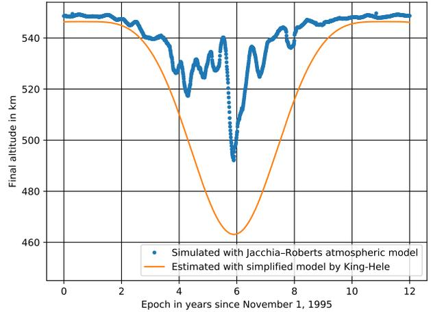
**Figure 4:** Loss of spacecraft altitude as a function of its deployment epoch/time, as evaluated by orbit propagation on GMAT with the Jacchia–Roberts atmospheric model (blue circles), and by the model proposed for TAT-C's OMM (orange line). Each blue circle presents the final altitude after 100 days starting from 550-km altitude. For each consecutive simulation, the epoch is increased by three days.
