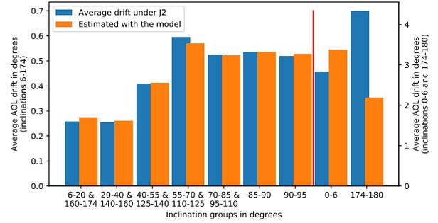
**Figure 3:** Average AOL drift rates due to  $J_2$  and as predicted by the model over five days. The validation data set is used here.
