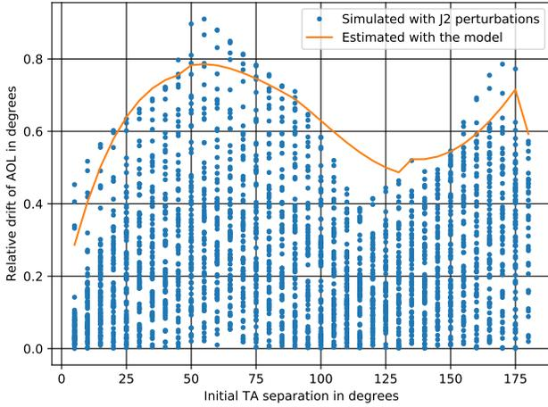
(b) Inclination of  $88^\circ$  and altitude of 419 km. Nine orbital planes with four satellites per plane.
