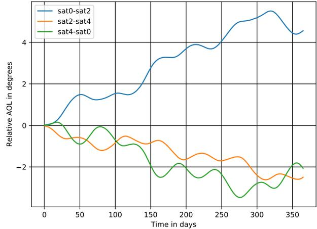
**Figure 8:** GMAT simulation results: The relative AOL drift between satellites in the three orbital planes of the TROPICS constellation.
