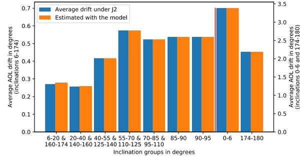
**Figure 2:** Average AOL drift rates due to  $J_2$  and as predicted by the model over five days. The training data set is used here.
