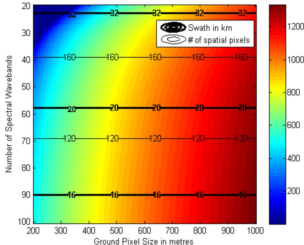
SNR at sensor for  $\lambda = 1010$  nm,  $\text{SZA} = 0$ ,  $\text{VZA} = 0$ ,  $h = 800$  km
