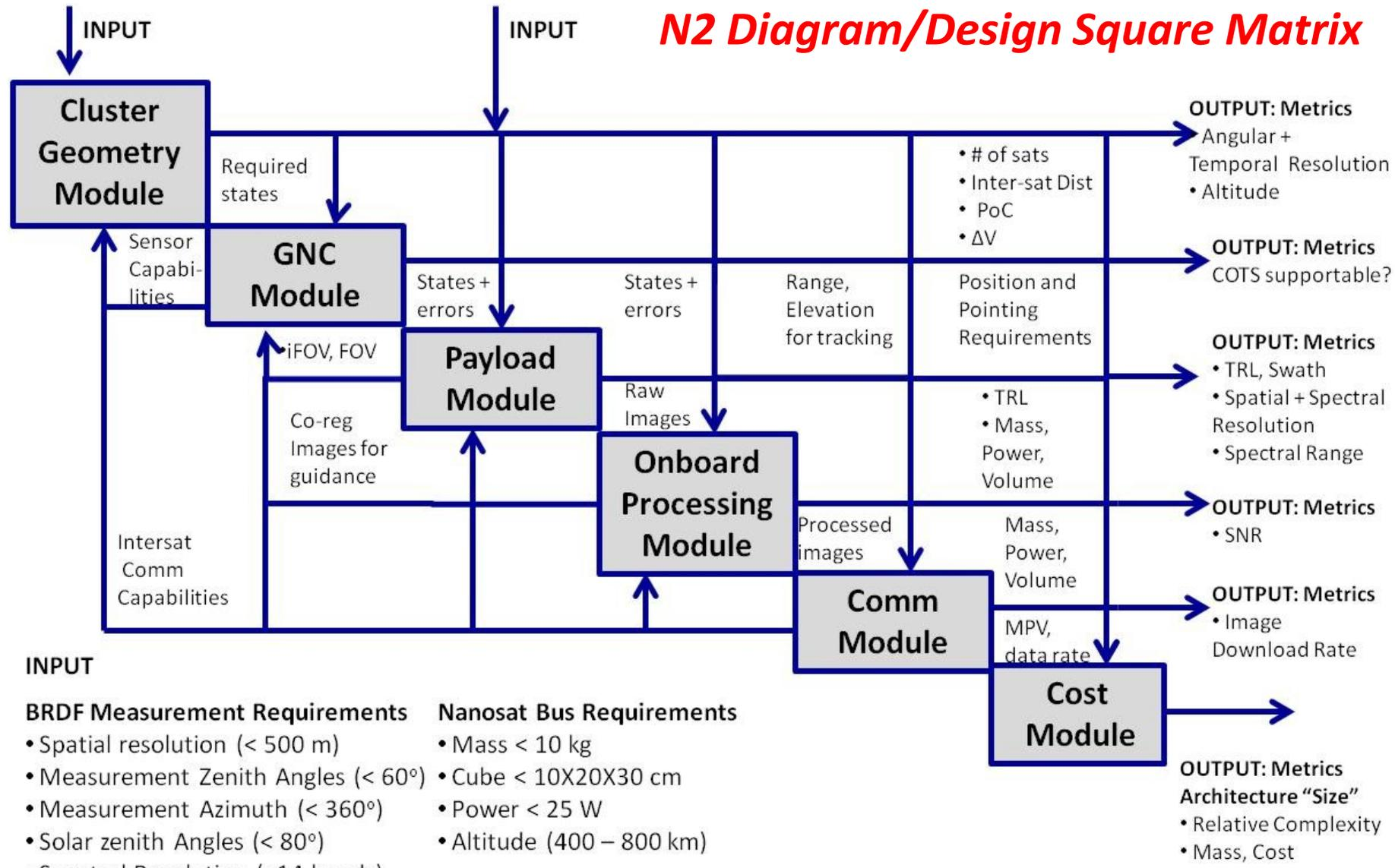
Preliminary design of a VNIR Imaging spectrometer for a nanosatellite to fit the BRDF spectral and spatial requirements
