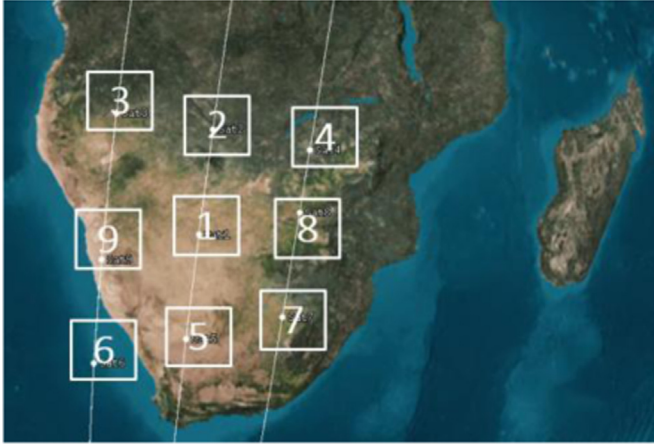
Fig. 10. 8 available differential RAAN-TA slots (exact values in Table 3) arranged around the reference satellite (+1), as enumerated in an AGI-STK simulation. At any instant, one satellite points nadir while the others point to the ground spot below the nadir-pointing, reference satellite.
