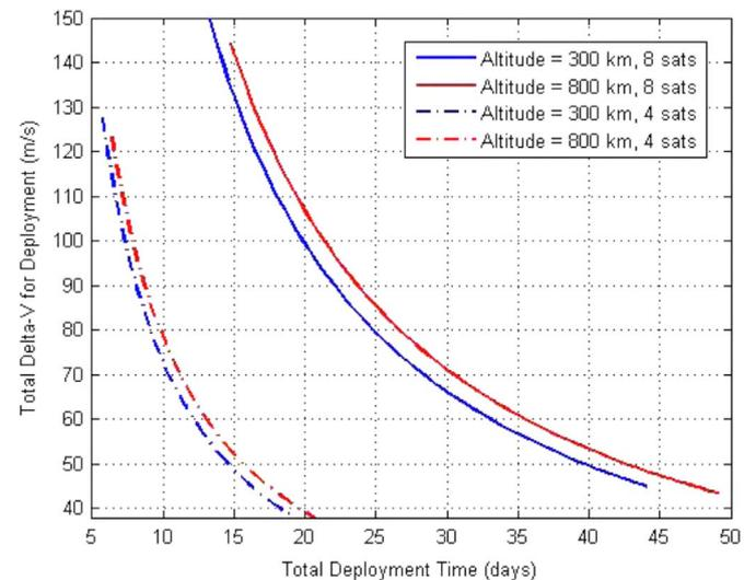
**Fig. 10.** Trade-off between total  $\Delta V$  (proxy for required fuel) and deployment time required to propulsively deploy 4 or 8 uniformly spaced satellites in the same plane. Time is a function of the phasing orbit.
