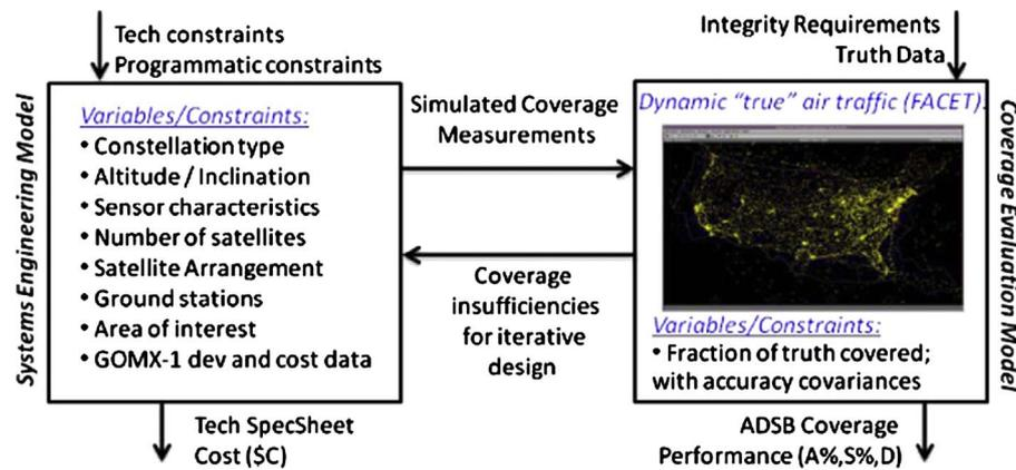
Fig. 1. Coupled constellation design (driven by Model Based Systems Engineering or MBSE) and evaluation (driven by science-inspired Observing System Simulation Experiments or OSSEs) tool for designing an air-traffic monitoring sensor network in space.
