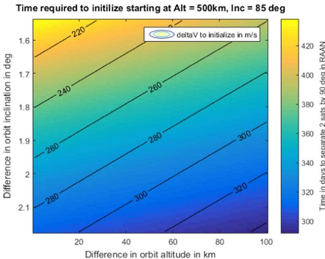
**Fig. 15.** Time- $\Delta V$  trade-off for moving 2 satellites from zero to 90° apart in RAAN as a function of differential altitude and inclination, using chemical propulsion. The colors indicate time in days and the contours are  $\Delta V$  in m/s. (For interpretation of the references to color in this figure legend, the reader is referred to the web version of this article.)
